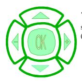
$\triangleleft$   $\triangleright$  This pair of keys is for scrolling the various symbols on the display, and, when a symbol has been selected, they are for choosing among the different alternatives (e.g. on/off) or setting new values.
